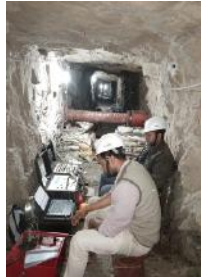
Fig. 8 - PJT in horizontal direction
