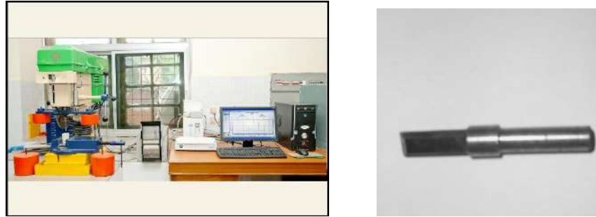
Figure 3 - Test setup for Siever’s J value determination
