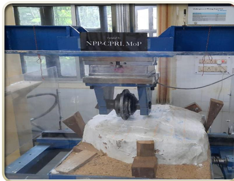
Figure 11 - LCR test setup with sensors and measurement parameters
