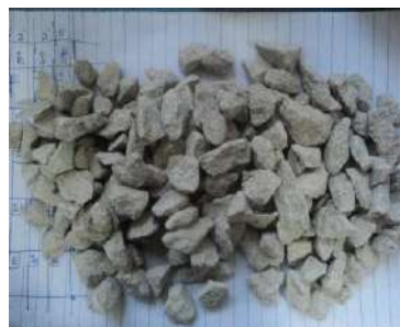
Initial sample of size between 11.2 - 16 mm
