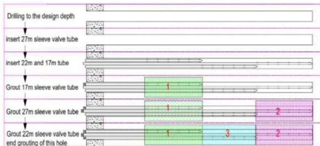
Figure 9 - Schematic stage grout injection (Nos. 1, 2 and 3) through a sleeve pipe (Figure not in scale)
