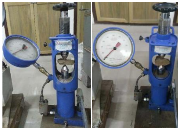
Figure 4 - Laboratory test setup for point load test
