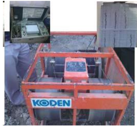
Fig. 26 - KODEN measuring device, KODEN output unit (top left), output (top right)
