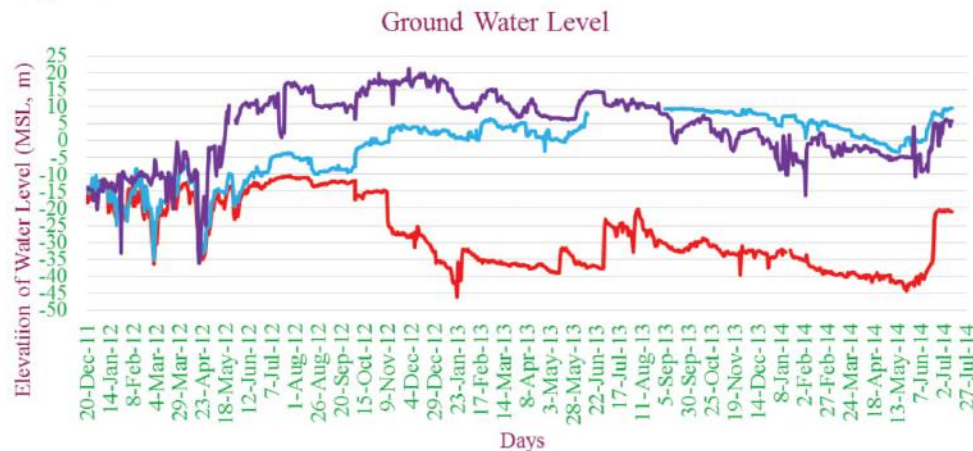
Fig. 12 - Recovered ground water level after grouting and additional borehole
