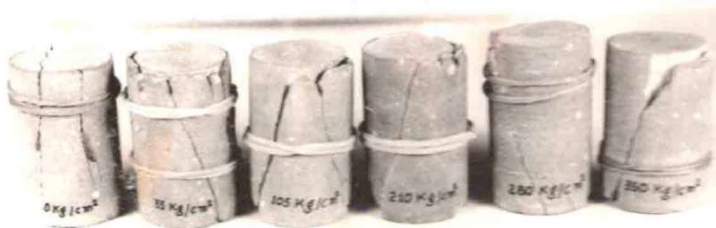
Fig. 8 – Failure under triaxial tests
