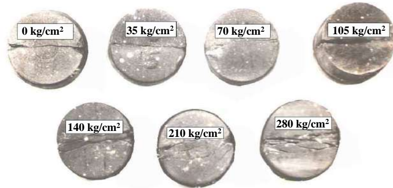
Fig. 7 – Failure under unconfined and confined Brazilian tests
