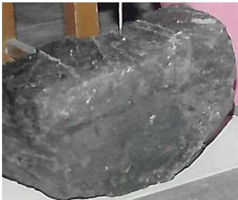
Fig.2 - Rock sample kept on specimen holder for determination of Joint Roughness Coefficient
