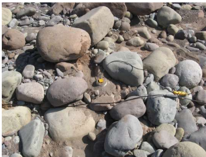
Fig. 7 - Arrangement to fix geophones in exposed bouldary surface
