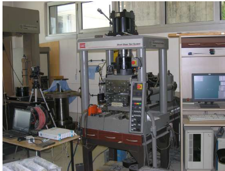
Fig. 15 - MTS machines used for direct shear, uniaxial and Brazilian tests
