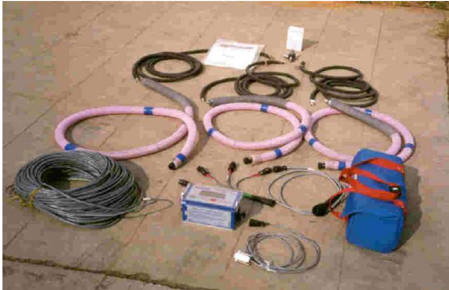
Fig. 1- Accelerometer based seismograph with accessories, Instantel Make
