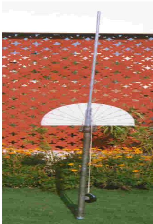
Fig. 2- Telescopic overbreak measuring rod (fabricated)
