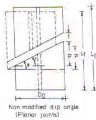
Fig. 9. Unmodification in dip angle for planar joint
