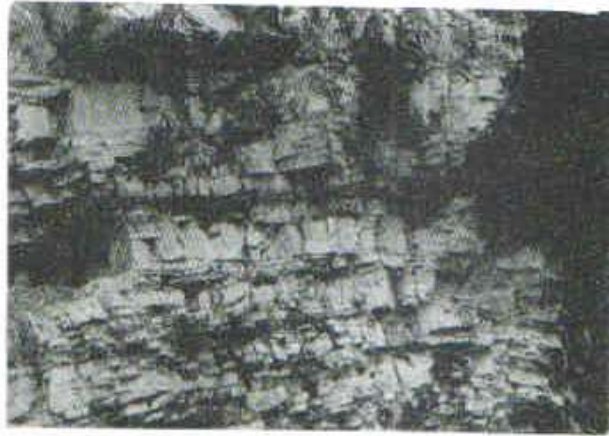
Fig. 1. Presence of gouge in rock joint
