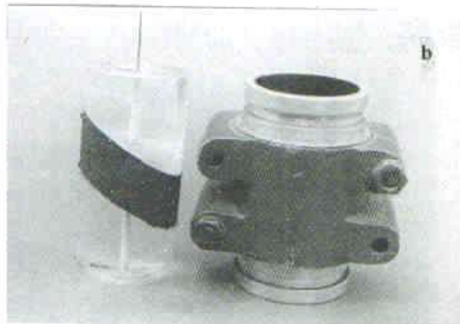
Fig. 6. (a-b) Typical Test specimens of infilled joints (undulating and planar type of joints)
