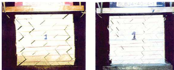
Fig. 7 - Typical specimens failed due to sliding
