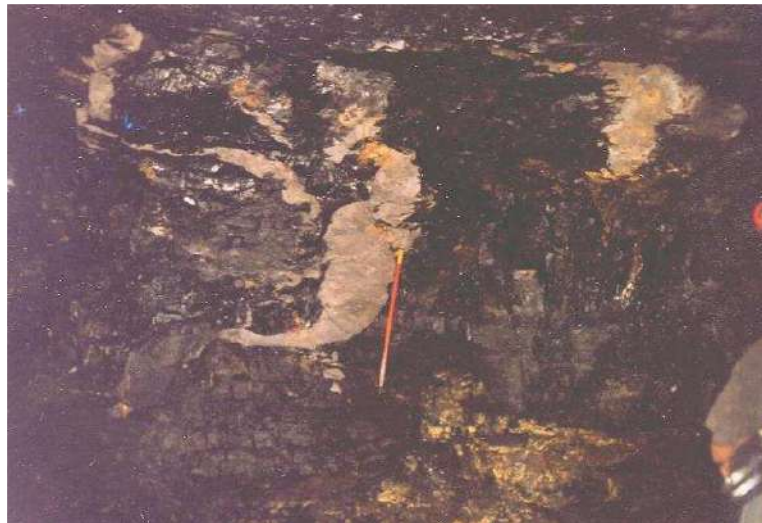
Fig. 3 – Sandstone dyke in the coal seam and roof of working section
