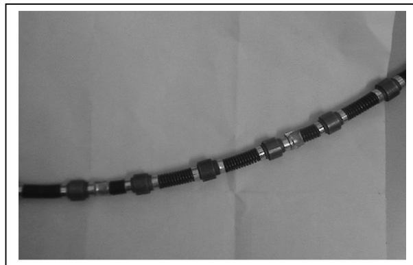
Fig. 3 - Diamond wire with 2000 number of beads
