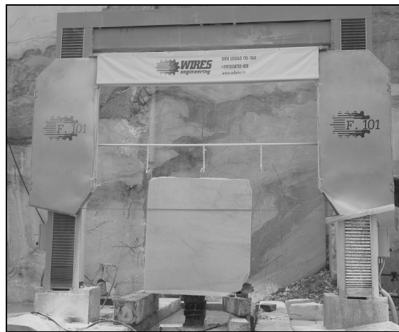
Fig. 4 - Single diamond wire block machine and cut surface of the block
