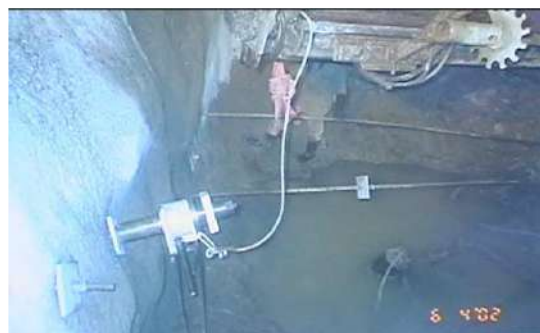
Fig. 4 - Set up of pull out test by Dywidag stressing machine
