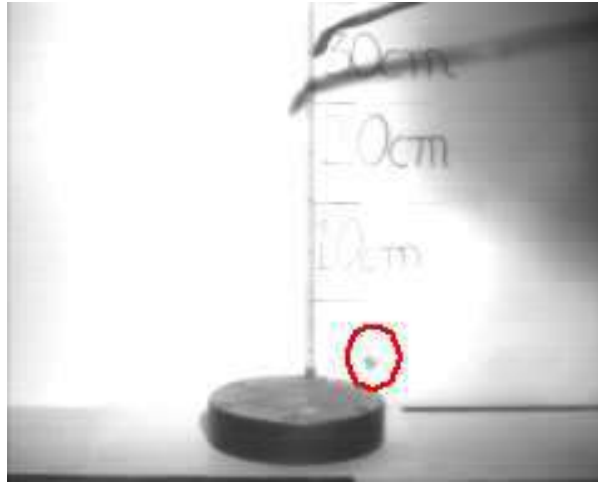
Fig. 8 - The limestone particle at the highest position after rebounding on the steel surface.
