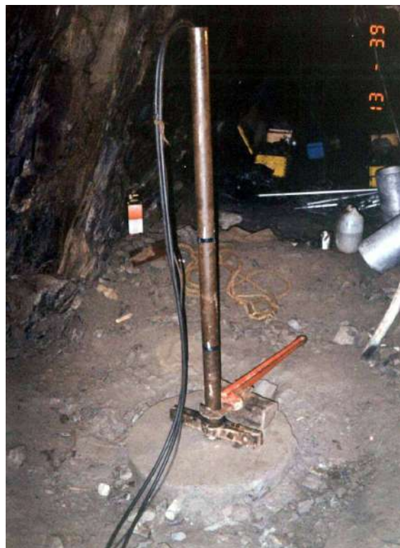
Fig. 4 - Goodman jack inside drillhole
