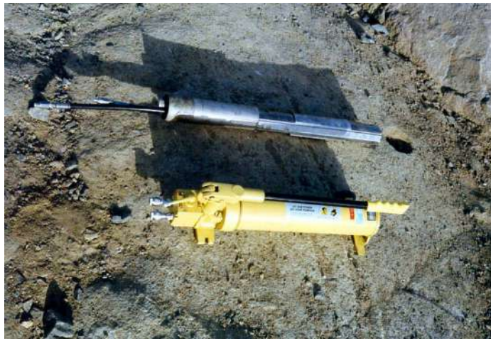
Fig. 3 - Goodman jack along with hydraulic pump
