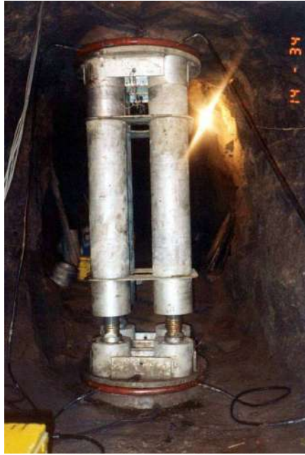
Fig. 7 - Plate jacking test loading assembly
