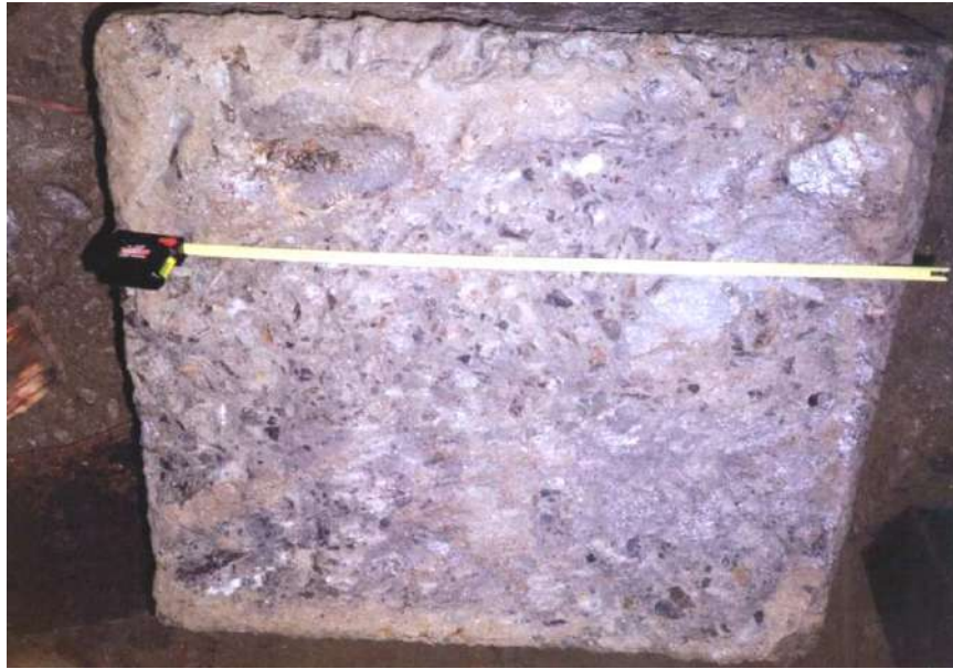
Fig. 6 - Measurement of shear surface for correct shear area calculation
