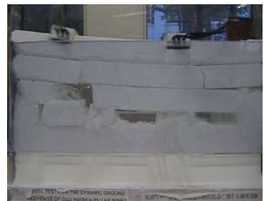
Fig. 6 - Some views of models of abandoned lignite mines during shaking table tests
