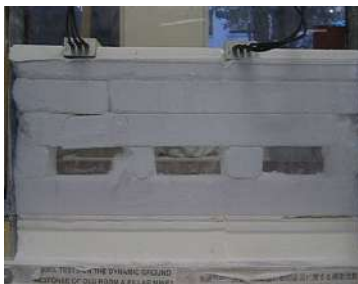
Fig. 6 - Some views of models of abandoned lignite mines during shaking table tests
