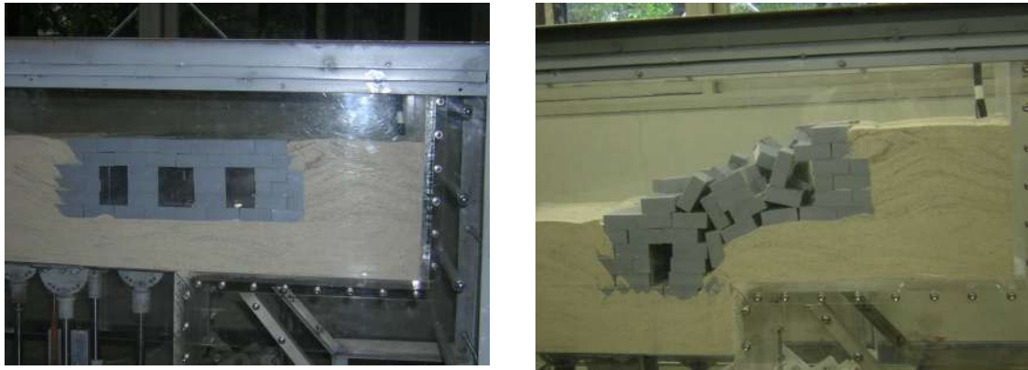
Fig. 7 - Views of damage to an abandoned room and pillar mine by vertical normal faulting
