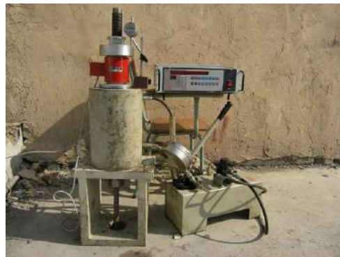
Fig. 2 - Pull out test components
