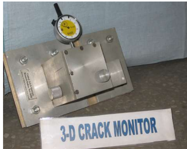
Fig. 5 – Three dimensional (3D) crack monitor
