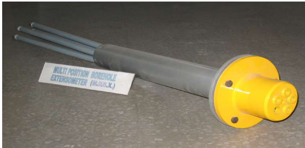
Fig. 6 - Multi position borehole extensometer (MPBX)
