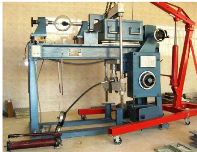
Fig.7 – General set-up of direct shear testing equipment
