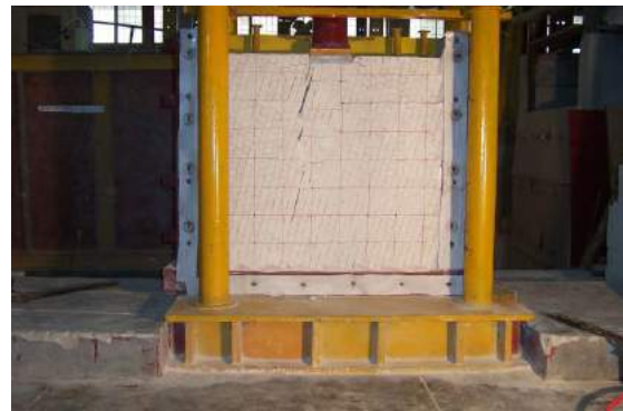
Fig. 6(f) - Failure mode in type-B specimen, 75°-15° ( \theta = 75^\circ , s = 0.5b )
