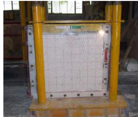
Fig. 5(b) - Failure mode in type-A specimen, 15^\circ-75^\circ ( \theta = 15^\circ , s = 0 )
