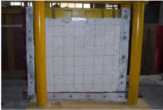
Fig. 6(c) - Failure mode in type-B specimen, 30°-60° ( \theta = 30^\circ , s = 0.5b )
