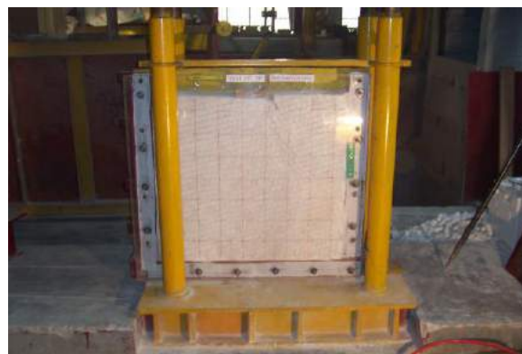
Fig. 6(b) - Failure mode in type-B specimen, 15^\circ-75^\circ ( \theta = 15^\circ , s = 0.5b )
