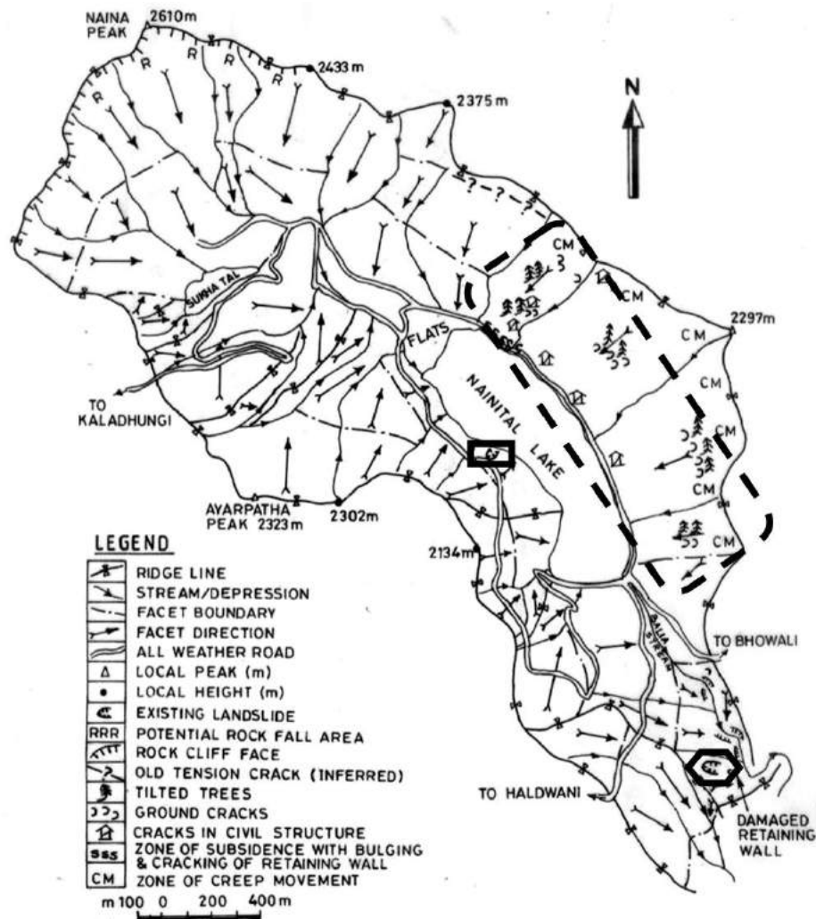
Fig. 5 - Ground Instability Indicator map of the study area. Note: Highlighted portions show the areas where evidence of slope distressing is most prominent
