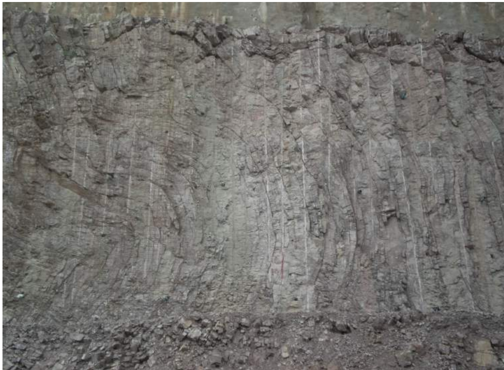
Fig. 2: Photograph showing joint and folding in the limestone of approach channel area
