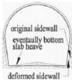
Fig. 6g - Bottom cracks and wall deformation
