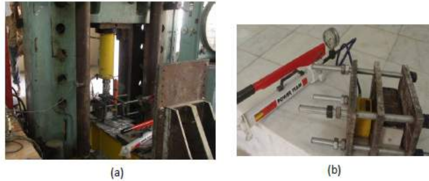
Fig. 2 - Test of samples under biaxial loading condition (a) hydraulic type biaxial frame (b) oil pressure pump system
