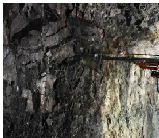
Fig. 5b - Dyke and hydrothermal alteration
