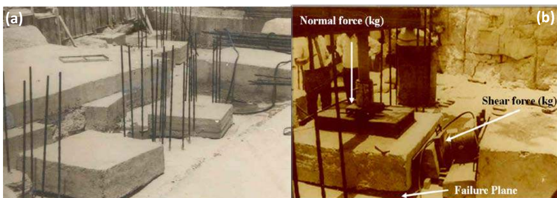
Fig. 2 - (a) Concrete capped rock blocks and (b) application of normal and shear forces on the test block at Rajasthan Automatic Power Project (RAPP) site
