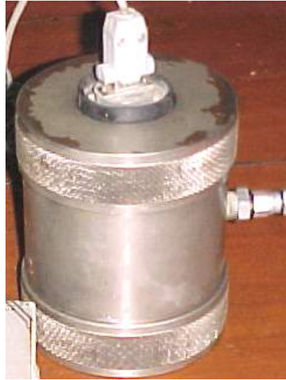
Fig. 8 - Cylindrical core containing the strain gauge device being loaded into bi-axial chamber to measure the Young's modulus of elasticity
