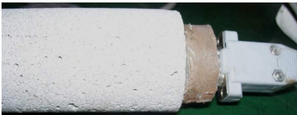
Fig. 7 - Cylindrical core mounted with SRB connected with interface cable through 9-pin 'D' connector
