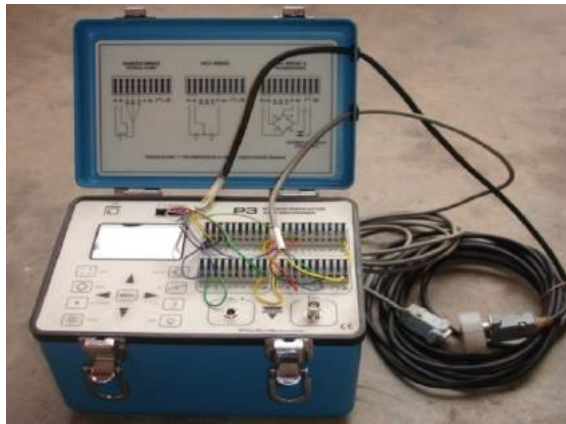
Fig. 3 - Portable strain recorder with 9-pin 'D' connector connected to the SRB
