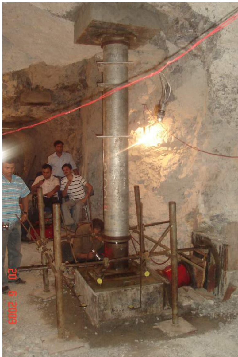
Fig. 4 - In situ shear test assembly inside drift
