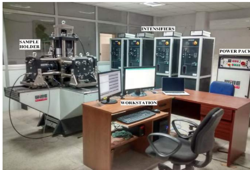
Figure 2: Polyaxial testing machine at IIT Roorkee
