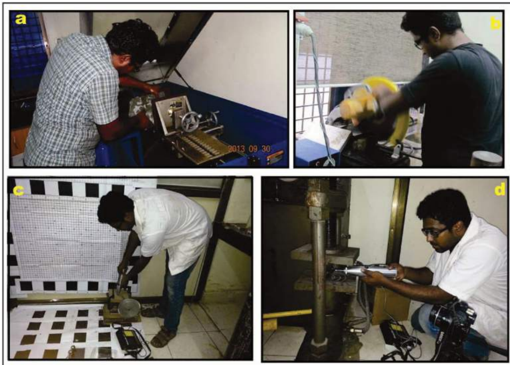
Fig. 1 - Preparation for laboratory experiment: (a) and (b) cutting and polishing of rock slab; (c) and (d) setup for measuring Schmidt hardness for slabs and balls
