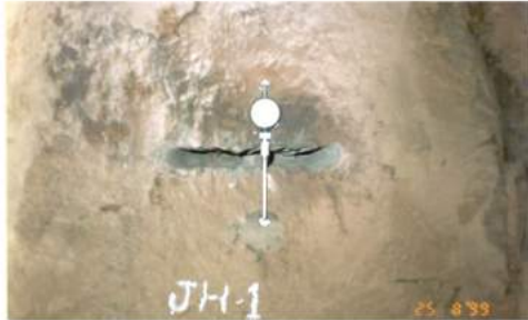
Fig. 5 - Measurement of distance between reference pins by deformer
