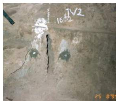
Fig. 4 - Slot cut in vertical direction to measure induced stress along the tunnel axis
